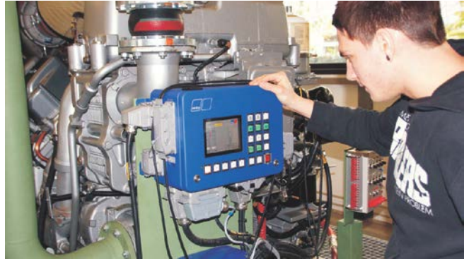
MTU Training station: Looking for a malfunction at the engine control equipment
