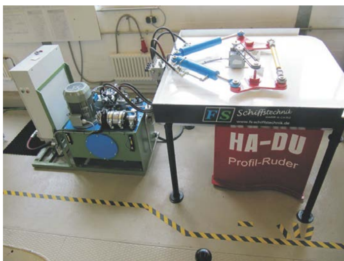
Rudder system to understand the function and to train maintenance tasks
